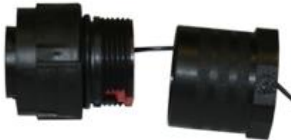
Screw the cable clamp into the back shell
