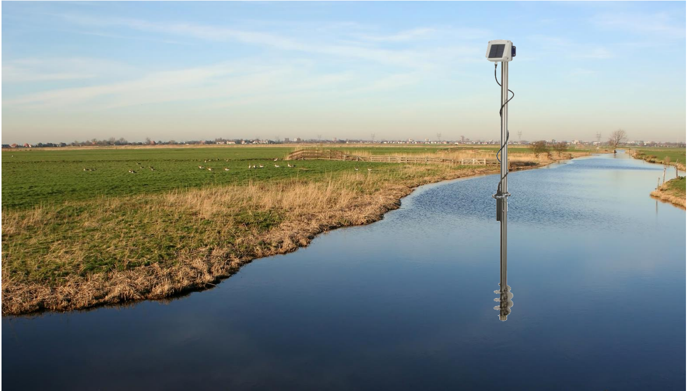
Compact measurement setup for online measurement of salinity
