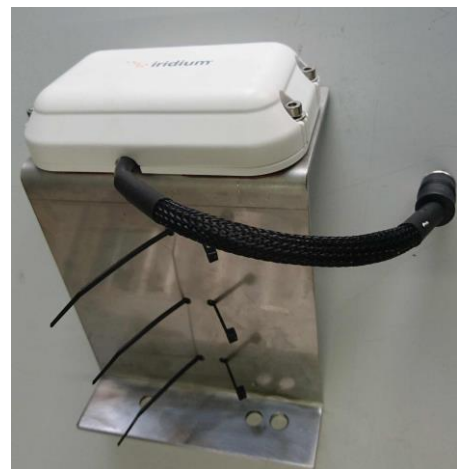
The OMC-IEM with its pigtail. Shown here mounted on a bracket.
