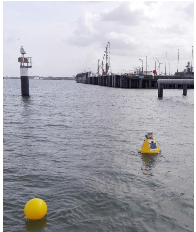
Application of the OMC-IEM in the OMC-7006 data buoy
