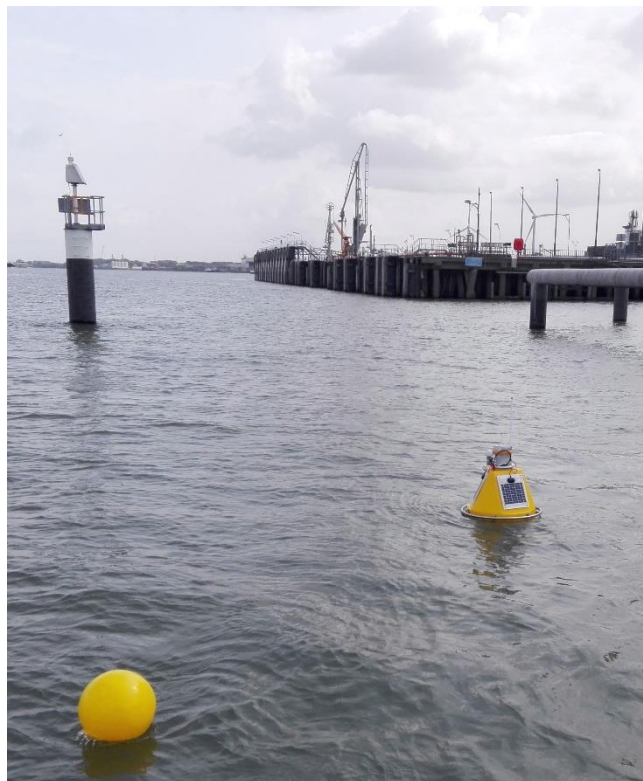
Application of the OMC-048 in the OMC-7006 data buoy
