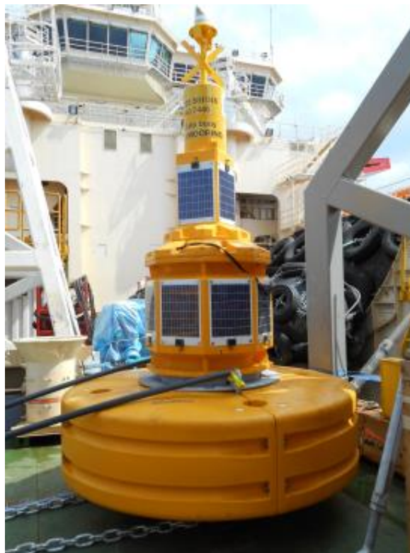
The instrument tower of the OMC-7018 mounted on a larger (2.4 m) float with 4 tubes for hydrological sensors.
