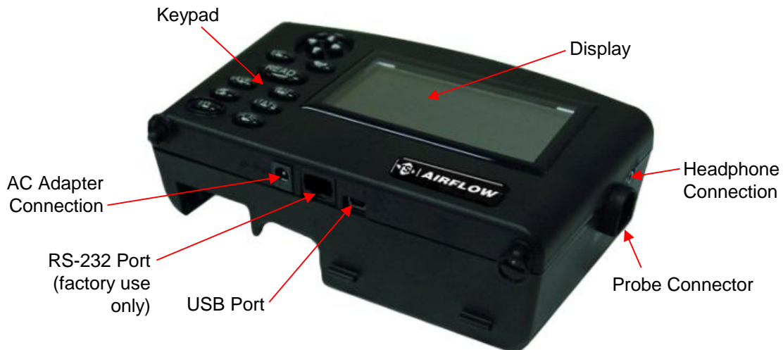
Figure 1: Features of the PH730/PH731 Micromanometer, Front View
