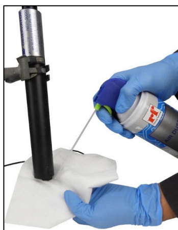
Figure 10.G: Dry the probe
