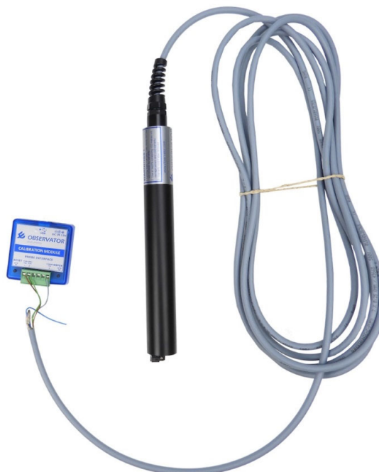
Figure 6.F: Example of configuration for SubConn SDI-12 probes
