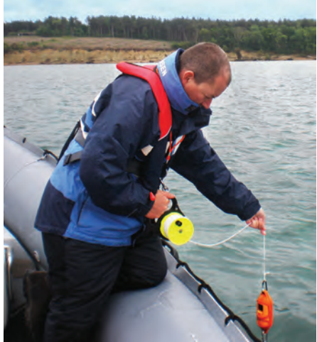
The CastAway is a multi-functional tool that incorporates the most modern technology available - yet is simple to use. It is designed for CTD profiling down to 100 m and is easy to deploy.
