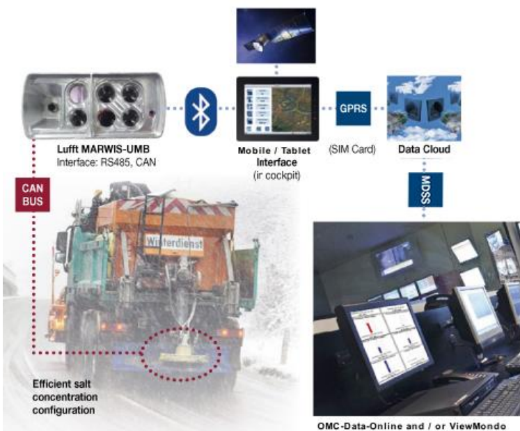
MARWIS - Mobile Road Weather Information Sensor
