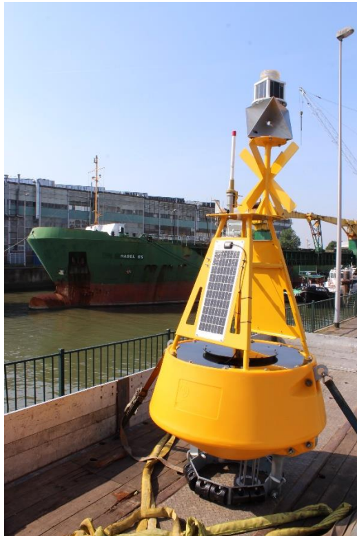
OMC-7012 data buoy, typical configuration
