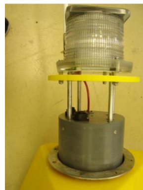
The contents of the water-tight container. The water-tight container slides from the top into the buoy.
