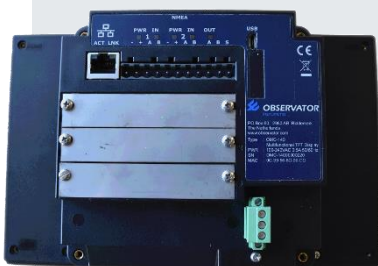
Screw terminals for power supply (green stands for AC and grey for DC)
