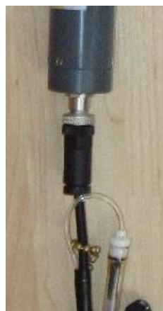
^ INW connector (IP67) installed on tube housing.
