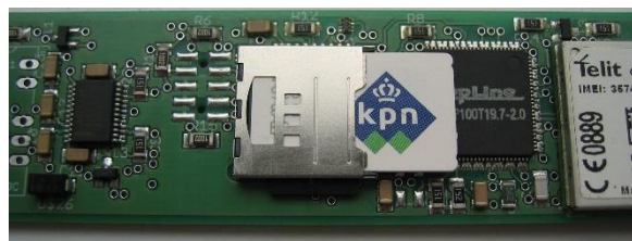
^ SIM card installed on PCB, 2 GB Micro SD memory card is positioned under SIM card holder.
