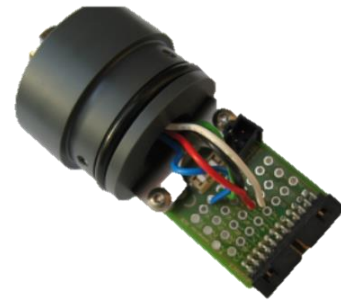
OMC-040 connection board with bottom part
