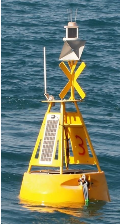
OMC-7012 data buoy for hydrological and meteorological sensors. Diameter: 120 cm.
